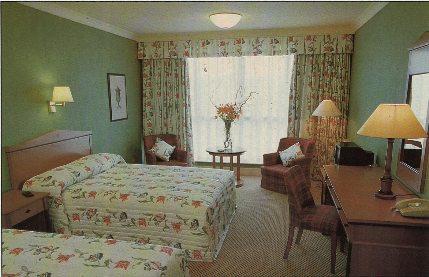
Forte Hotel: The bedrooms are lit by wall lights and table lamps using PL13 compact fluorescents; the ceiling fittings take two such lamps.
